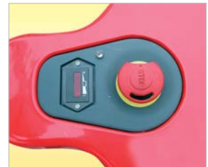
Emergency stop button and voltage gauge conforming to human dynamics.
