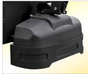
Robust metal shell protecting electric motor and wheels avoids hurting of foot.
